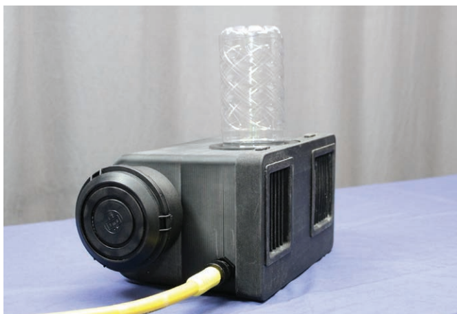
© Fraunhofer USA, Fraunhofer USA created heat and humidity unit for Neonatal Intensive Care Incubator.
